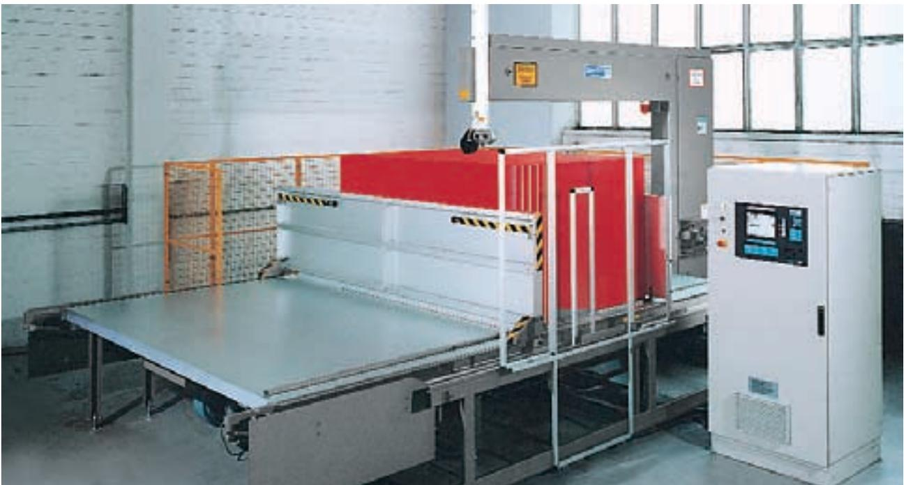
Fully Automatic Vertical Cutting Machine V 51
