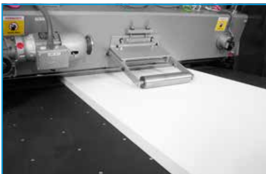
Splitting Machine H 24 G with optional feeler roller
